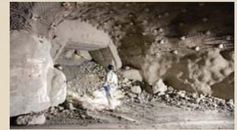
A 'block' of ore is undercut to initiate caving, whereby gravity is used to make ore 'cave' under its own weight. The undercut zone is drilled and blasted progressively and broken ore is drawn down to create a void into which initial caving of the overlying ore can take place.
